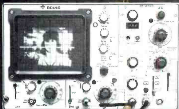
Gould's monitor/oscilloscope can display a complete picture with a bright line indicating the line under examination.
