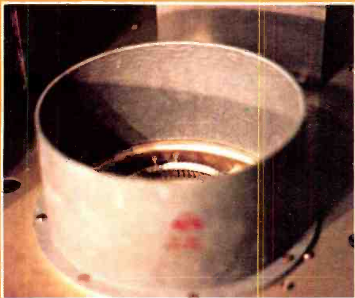
(c) The new EIMAC type SK-1306 chimney in place.
